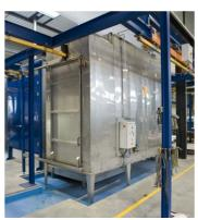
After treatment the parts are coated by a 1-2 micron thickness organic coating which can *increase the top coat adhesion,* provide a temporary protection of some weeks if parts are stored inside, and **increase corrosion resistance on steel with powder coating up to 400-500 hours** or even more in salt spray (specific test must be carried out)..
