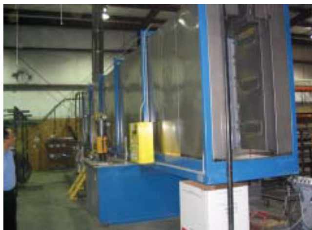
An in-line flowcoat tunnel used to pretreat lighting fixtures for the hospitality industry. The tunnel is 41 feet long, with a line speed of four feet per minute. Polyethylene curtains at the entry and between zones control air flow.
