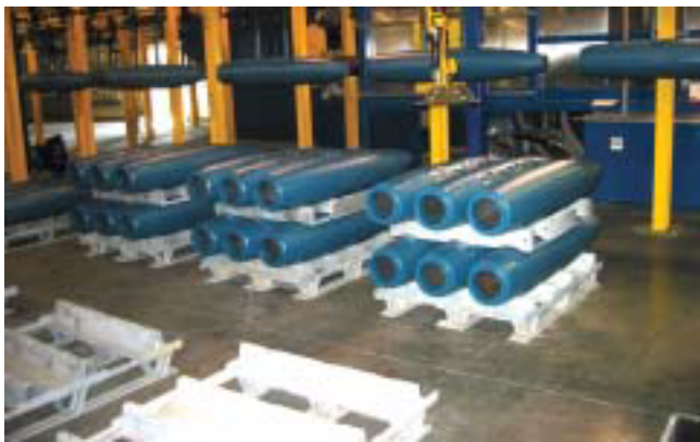
An in-line flowcoat installation in operation, making casings for test bombs. The one-step phosphating system has Mil. Spec. approval.
