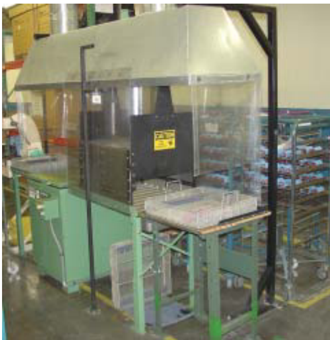
A small, self-contained dip unit for treating motor armatures. On the left is the dip tank in which parts are treated and dripped off. Then the parts are blown off (middle section) and staged for powder coating.
